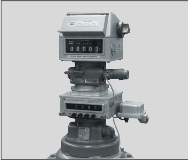
through drive from the gross meter output to gross register or accessories. The extension length should be specified based on height necessary to clear the net accessories. From the standpoint of mechanical limitation, the dual head ATC has 1% greater maximum temperature range than meter ATC. Mechanical range and limitations are indicated by lines A-A", Figure 4.
